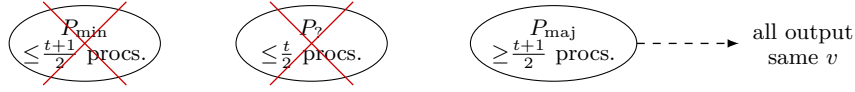
■ Figure 1 Execution E_{\text{crash}} , where processes of P_{\min} and P_? crash, and only processes of P_{\text{maj}} stay correct, which leads to a safety violation.
